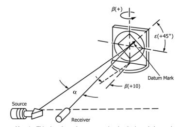
Note 1—This view shows the source-receiver in a horizontal plane and the entrance angle  $\beta$  (=  $\beta_1$ ) as a rotation about a vertical axis. The rotation angle  $\epsilon$  is shown at +45° for illustration purposes— default position is  $\epsilon = 0^{\circ}$ .
